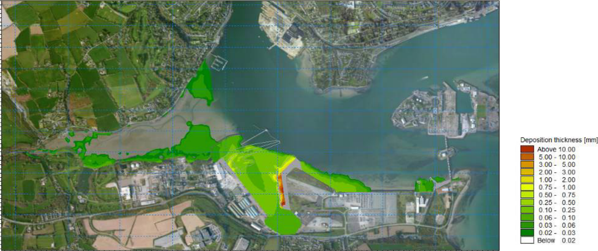
Figure 12.18 Final Sedimentation following permitted development Dredging Operations
